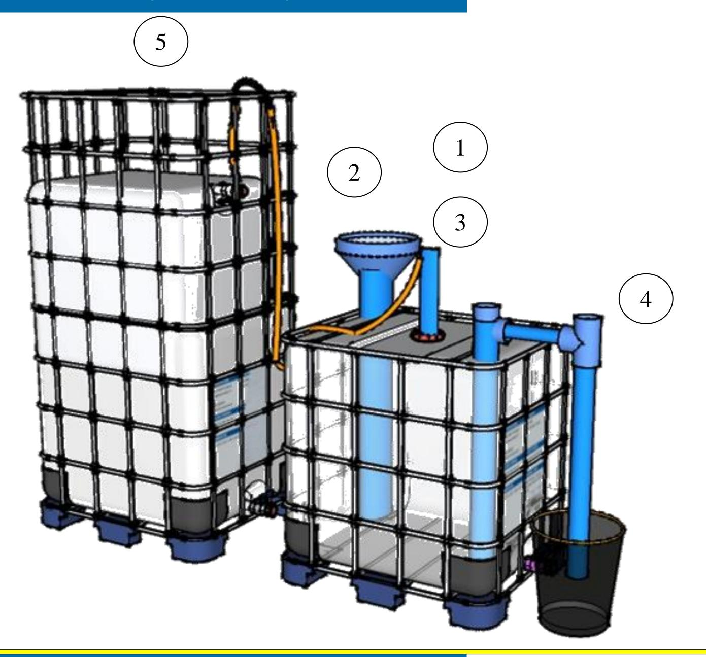
Three 1 m<sup>3</sup> IBC tanks are the base for the reliable and cost-effective Solar C<sup>3</sup>ITIES biodigester system. Both fermenter and gas storage are included and are dimensioned to cover the daily needs of gas for a small household.
