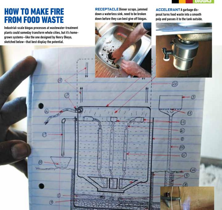
**DIGESTION** Microbes inside the 500-gallon tank break down the waste, giving off methane gas.
