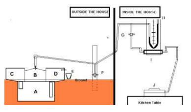
important to allow for maximum generation of biogas. The mixing happens as the slurry moves forward and backward between the AD tank and the DT tanks. A schematic is presented in the figure.
