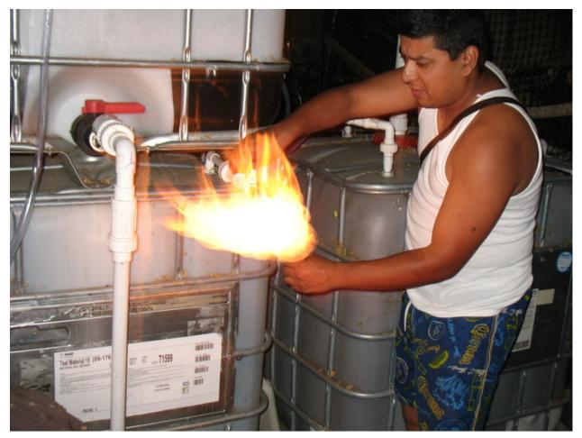
Figure 27. Figure showing how gas is piped from digestor to collector
