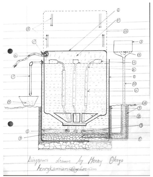
Figure 19. Figure shows a schematic of the digestor we built with Simama e.V. at the Mukuru School in Nairobi, done by teacher and plumbing specialist Henry Okeyo Kamiseria (who is now the local biogas expert
