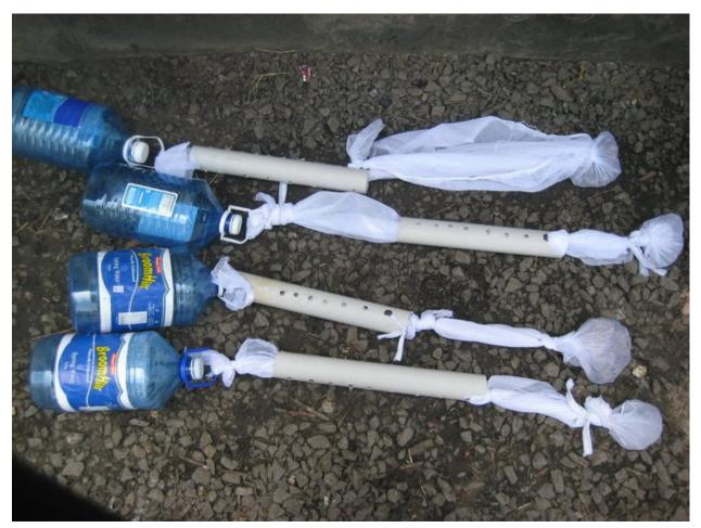
Figure 16. Another experiment for placing the bacterial fuel rods was conducted in the Mukuru Slum in Nairobi by our Solar CITIES interns Minke Noordam and Nils Andersch, art instructor Dave Redmond and teacher Henry Okeyo. In this case they suspended the rods using plastic bottles and weighted them with stones .
