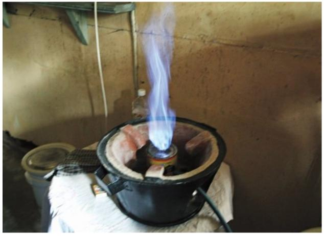
Figure 6. At the Jamhuri Energy Centre, which develops local alternative-energy systems, Elizabeth N. Kimonge and Dominic Kahumbu Wanjihia build hybrid clay stoves optimized for biogas that can also use traditional wood or biochar fuels. The biogas is piped into a removable coffee can filled with stones with a peforated lid. When the gas runs out the coffee container can be simply removed and biomass put in to continue cooking.
