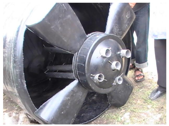
Figure 14. To use bacterial fuel rods in a completely plastic tank, In Nigeria we decided to insert the "fuel rods" into the cover of the tank with nail-pins on either end to allow them stay submerged as the gas collector rose and fell, sliding past them.
