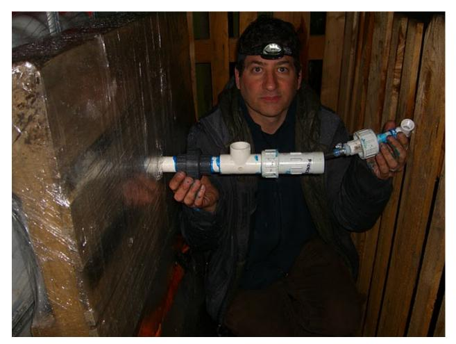
Figure 33. The heat exchanger plumbing
