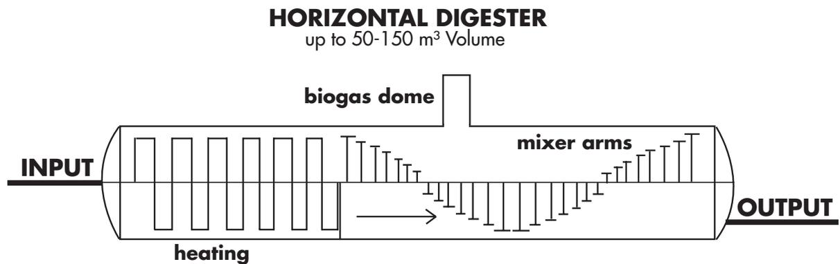
Plug-flow digesters are the simplest form of anaerobic digestion. It is the least expensive and is typically used in small farm projects. A plug flow digester is typically long and narrow, five times as long as it is wide. Plug flow digesters usually digest raw livestock manure. Plug flow digesters are less efficient than a traditional complete mix method. The benefit of a plug flow digester is reduced upfront capital costs.
