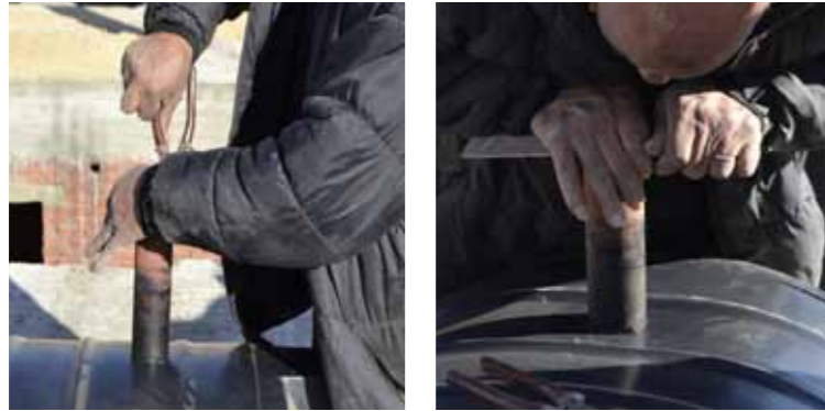
Fig.I_09: Clip a lower hole on the side of the bigger tank, using a hot metal pipe (2" in Diameter)
