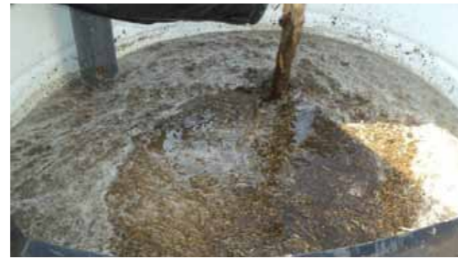
Fig.5_29: Mixing dung with water after filling the tank with them (taken by: Heidi Fink)
