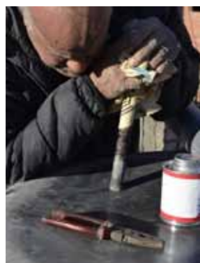
Fig.I_15: Cut a third hole, this time, at the bottom of the smaller tank (for the gas exit), use the same materials as before
