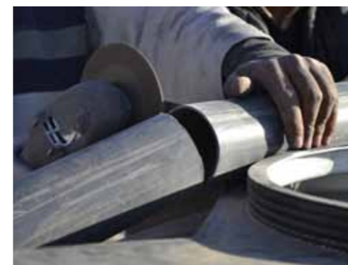
Fig.I_07: Cut the 3” pipe to the needed length
