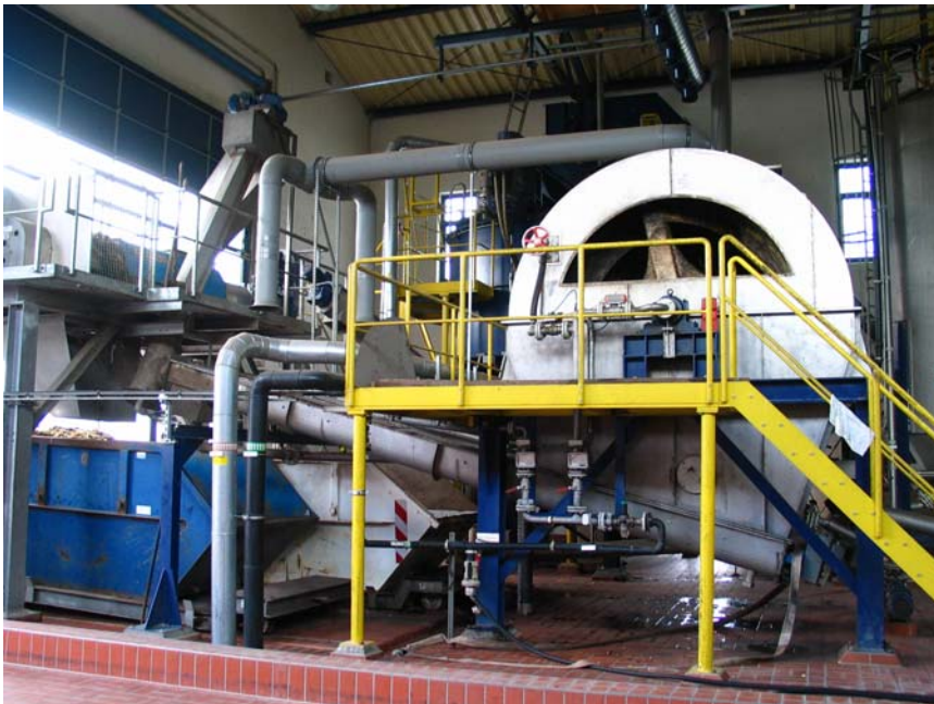
Figure 8.1-13: Machinery for mechanical processing of solid biowaste, market waste, etc. (Comminution, pulper, sieve for removal of disturbing particles).
