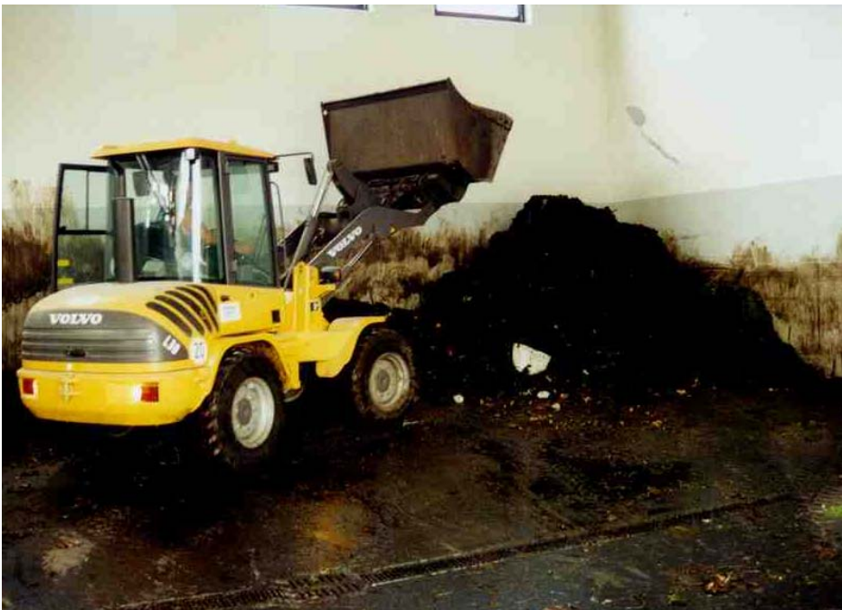
Figure 8.1-15: Bunker, with wheel loader and biowaste from communal waste collection.
