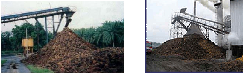
Figure 7.2-1: Generation of empty fruit bunches (EFB) in the palm oil industry
