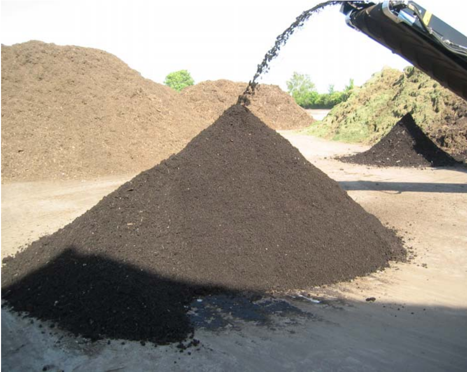
Figure 8.1-28: Sieving of the compost to a particle size of < 12 mm
