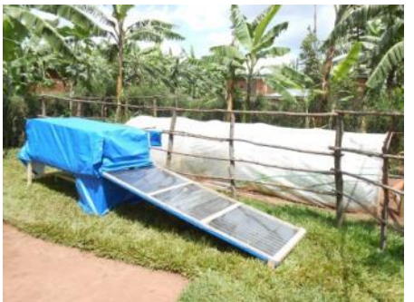
Biogas-Solar Combo Dehydration
