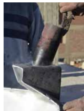
Fig.I_06: Use a hot metal pipe to hole the pipe space (3” in Diameter)
